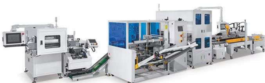
全自动包装+开箱+装箱+封箱(可定制化产线) Non-standard automatic packaging whole line
